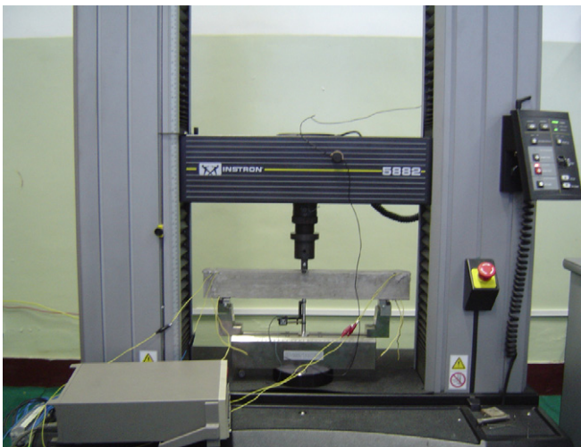
Fig. 7. Three-point load experiment setup.
